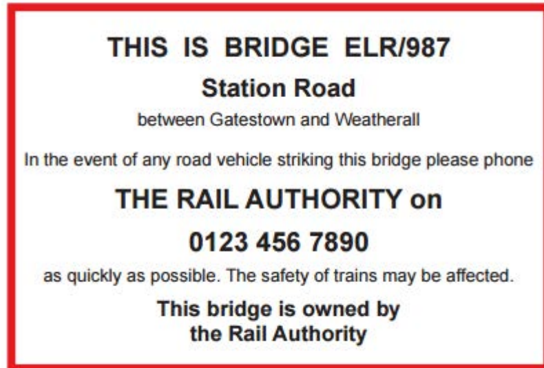
Example identification plate at a Network Rail bridge
